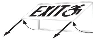
Faceplate slides up and outwards for quick and easy installation.
