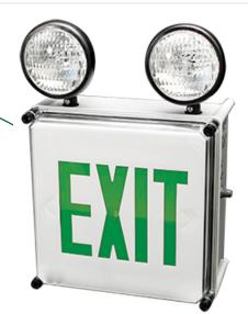
■ The durable **N4X-EPX** Is constructed from durable, corrosion resistant fiberglass. The NEMA 4X housing is fully gasketed for damp and wet locations with a hot-bonded silicone gasket.
