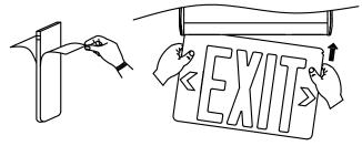
Insert fixture into hanger bracket and snap by spring, connect test switch, assemble LED indicator on bushing at trim plate. fix trim plate on the metal box by 2 screws.
