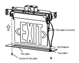
Determine direction for chevron indicator. (See DETERMINE DIRECTION)
