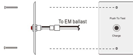
B. Install test switch on fixture surface.
