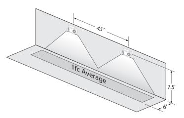
SAMPLE PHOTOMETRICS: M5-HO-U Using multiple M5-HO-U units (1.8 Watts lamps) mounted at a typical 7.5' height delivers 45' on-center spacing with a 6' wide path of egress.
