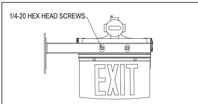
2. Attach conduit to hub on the fixture, making sure that at least five full threads are engaged and conduit is tight as per the requirements of the NEC.
