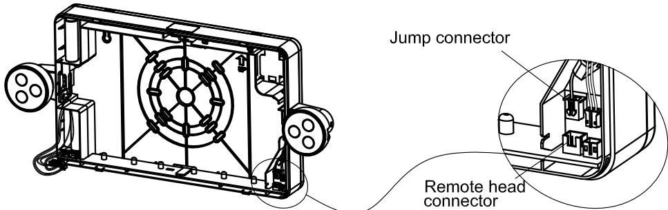
(2) Attach the remote male connector into the female connector on PC board.
