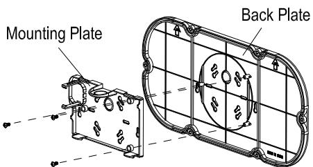
4. After install emergency lighting , assemble clear cover.
